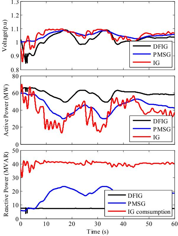
Fig. 7. Simulated responses to a measured wind speed. Starting from above: Terminal voltage, Active power output and reactive power output. The meaning of the curves is indicated in the graphs.
