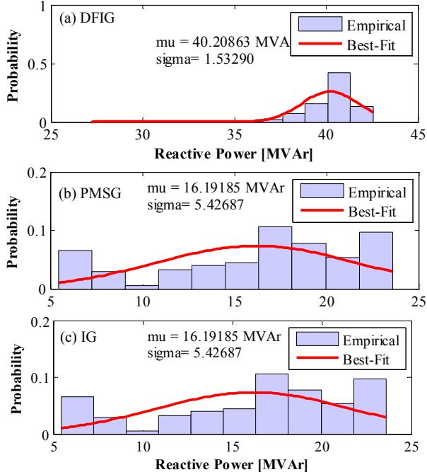
Fig. 9. PDF of the reactive power output for the considered WT.
