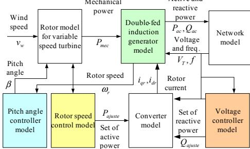
Fig. 3. General structure of tems VSWT using DFIG including the subsets and and their interactions [1].
