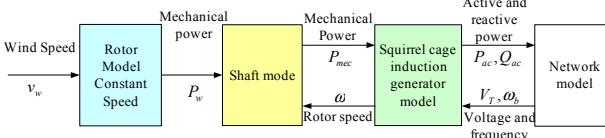
Fig. 2. General structure of tems FSWT using SCIG including the subsets and and their interactions [16].
