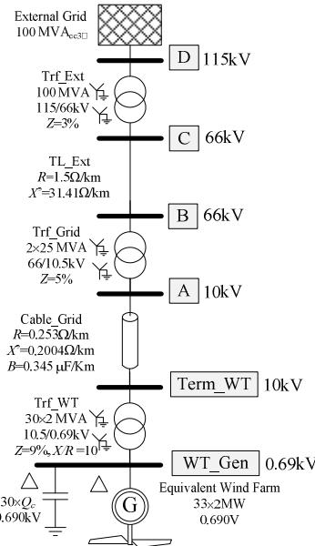
Fig. 6. Single-line diagram for the representative test system. Data of all components is depicted in the diagram.  $Q_c$ : variable reactive power compensation.
