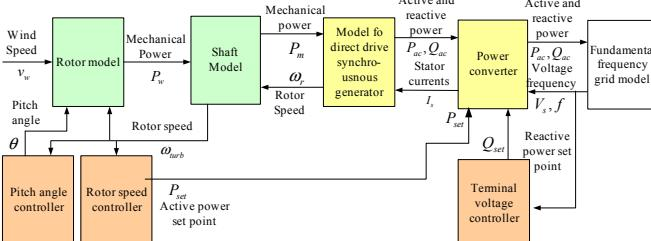
Fig. 4. General structure of typical VSWT using SG including the subsets and and their interactions [1].
