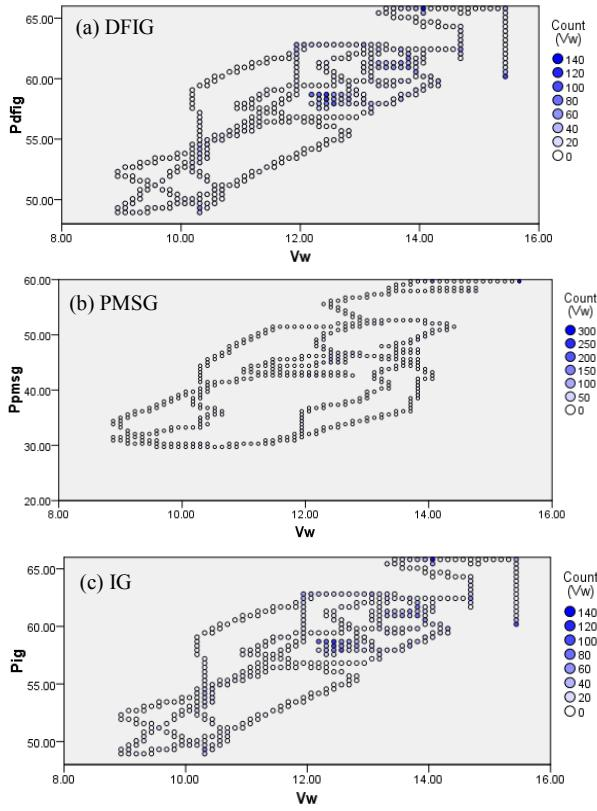
Fig. 11. Scatter-plots of active power output versus wind speed for the considered WT.
