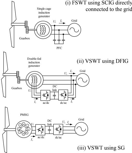
Fig. 1. Generating systems used in WT.
