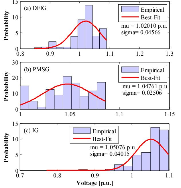
Fig. 8. PDF of the terminal voltage for the considered WT. The empirical and normal PDF are plotted for each one of the considered. It is not a primary objective of this paper to discuss about the fit goodness, otherwise conclusions about the variability on the electrical variables is the main concern.
